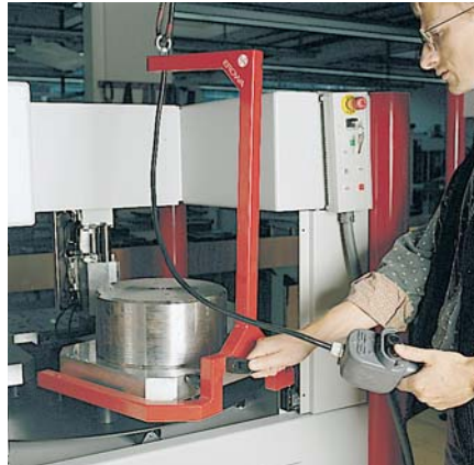
LiftGear UPC helps to change workpieces quickly, accurately and simply.
