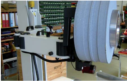
We also supply special grippers, for instance for the handling of large grinding wheels.
