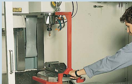
LiftGear UPC , for easy loading of the UPC chuck by means of an overhead crane. For information, please refer to page 290.
