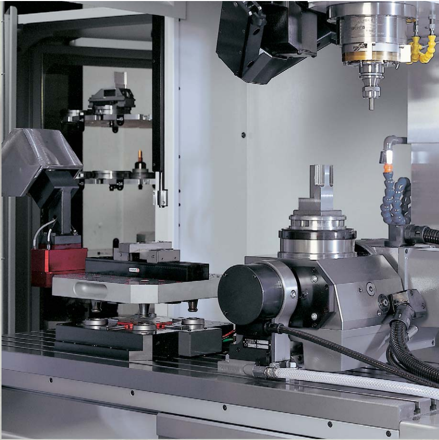
Flexible and automatic loading of a machine tool with an EROWA handling unit. The ratio of productive hours is considerably increased.
