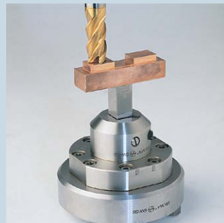
2. Milling On a straight System Plus holder.
