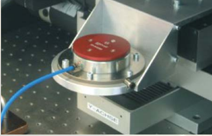
The cover prevents penetration of chips and dirt into the FTS chuck.
