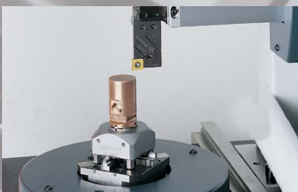
Setting-up and measuring outside the machine: quickl, simple and accurate.
