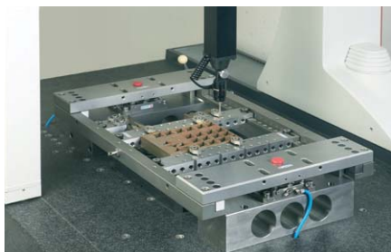
PreSet 3D CNC – presetting made easy. While the WEDM center is in operation, the next job is being preset quickly and accurately on the EROWA PreSet station.
