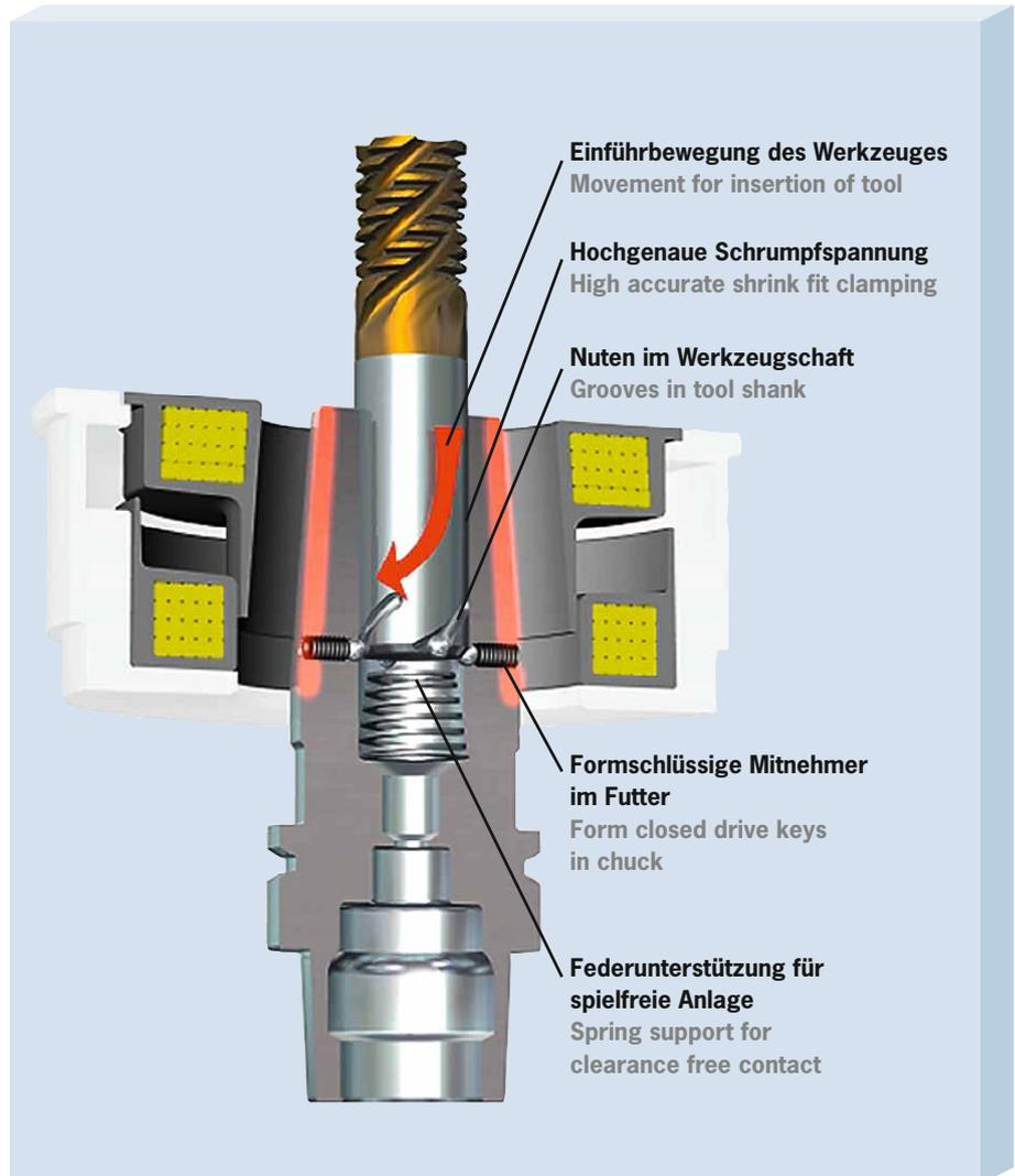
In high performance cutting (HPC), it is possible for the cutting tool to become pulled out from the chuck. The cause of this is a slow micro-creeping motion. It happens with cutting at high speed and with high pull out forces. Even chucks with extremely high clamping force cannot prevent micro-creeping. **High-quality workpieces become scrap as a result.**
